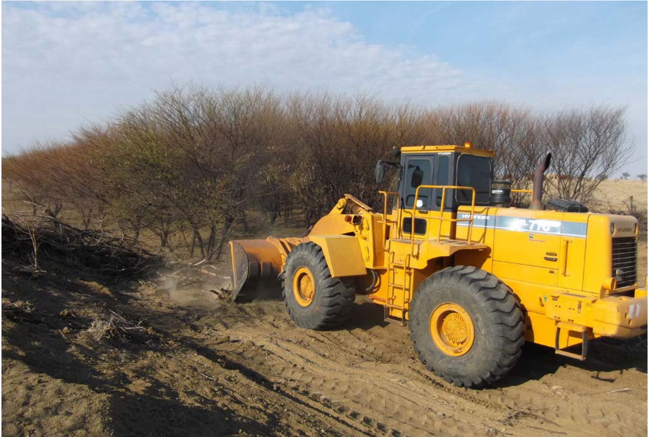
Figure 10: Loader pushing within a watercourse provided benefits of easier monitoring and follow-up control
