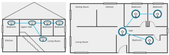
For HAS clients, HAS is able to replace smoke alarms not working or more than 10 years old with photoelectric alarms compliant with current Australian standards. An existing hard-wired alarm must be replaced with a hard-wired photoelectric smoke alarm.
